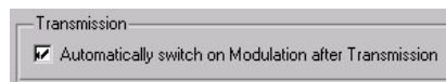
Fig. 7-11 To activate the burst control immediately after list transmission, “Automatically switch on Modulation after Transmission” in the “Preferences...” menu should be check marked.
